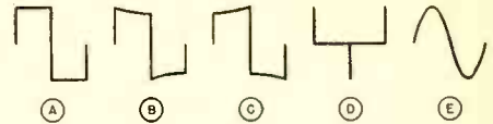
Figure 4. Various square-wave forms. "A" is perfect square-wave. "B" and "C" show low-frequency phase shift; "B" is poor low-frequency response, and "C" is high response at low-frequency. "D" shows extreme low-frequency attenuation, while "E" pictures a high frequency attenuation
